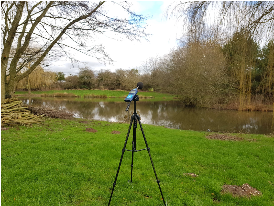
Picture 1: Noise measurement conducted with a class 1 sound level meter
